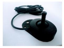
Stem type analog stick: Actuation force measured = 60 grams
